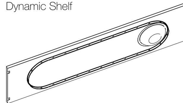
The dynamic shelf is the structure's most innovative part. It consists of a lamellar wood top that contains, although only a few centimetres thick, a motor that rotates the belt (on which the garments are hung) backwards and forwards. As the belt rotates, the garments, hung on any kind of hangers, also rotate, which allows their owner to see them without having to move around.
